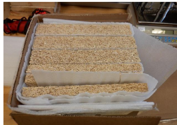
Cementitious Wood Fiber Acoustic Panel - 1" Thick, (Sample 1)
