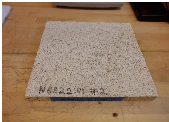
Cementitious Wood Fiber Acoustic Panel - 1" Thick, (Sample 2)
