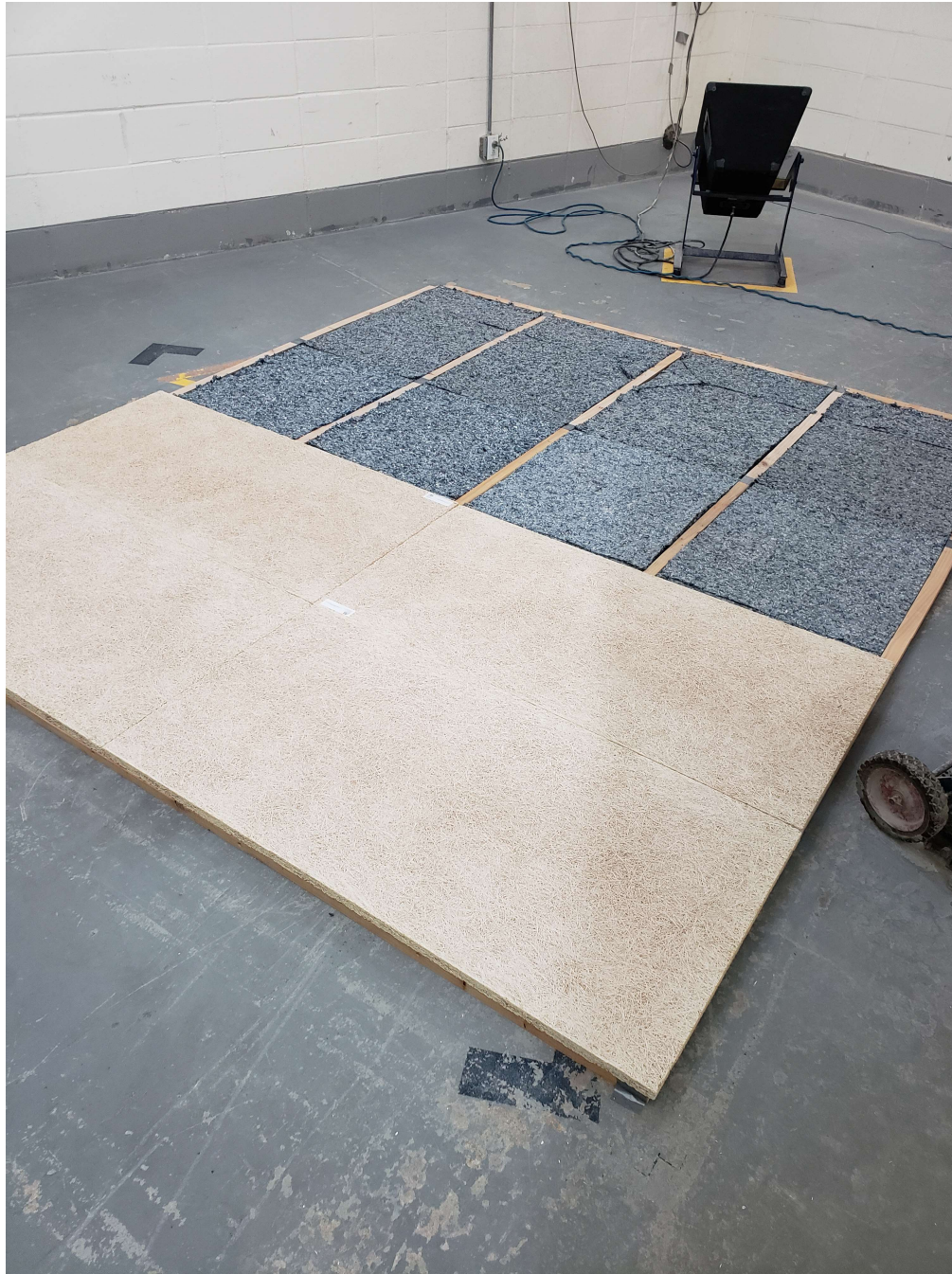
1" Cementitious Wood Fiber Acoustic Panel (C50 Layout)
