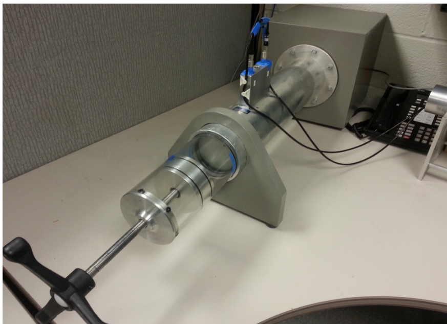
Sample Installed in ASTM E 1050 Test Fixture with 4" Air Space
