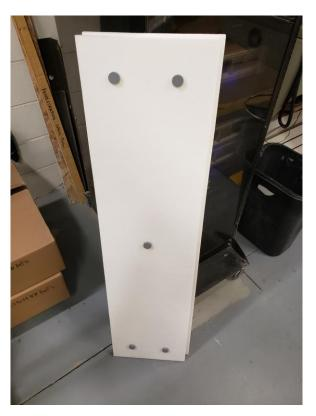
3D Printed Spacer Block (6mm Thick x 1" Diameter)
